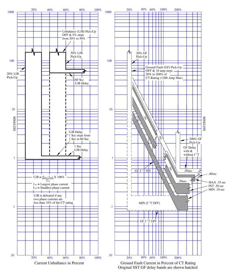
AC-PRO® ECS/SST Direct Replacement Current Unbalance & GF Time-Current-Curves
